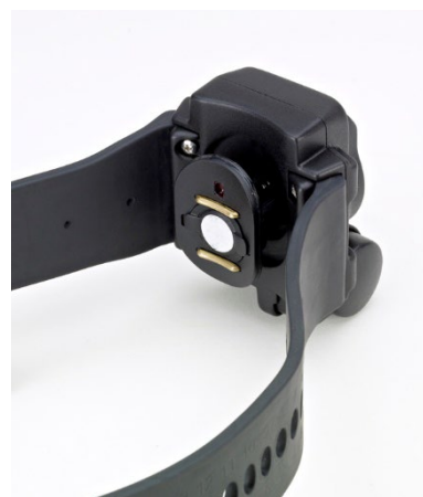
Figure 18. Alcohol Detection Sensor The alcohol Detection Module (ADM) samples the alcohol content of the client's perspiration to determine the client's TAC level.
